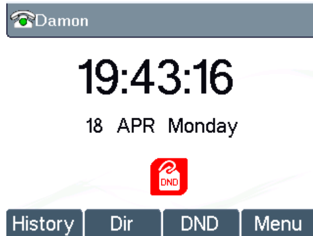
Figure 46 - DND Enabled on All Lines
