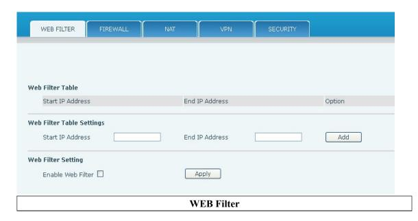
The Web filter is used to limit access to the phone. When the web filter is enabled, only the IP addresses between the start IP and end IP can access the phone.
