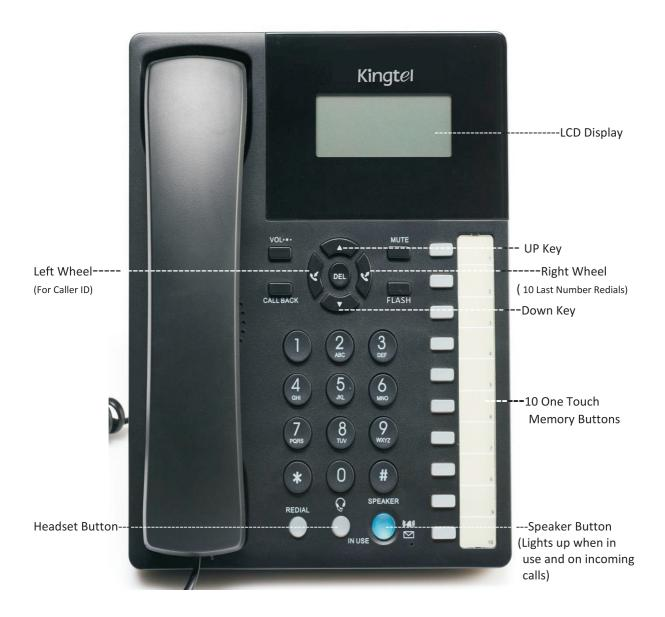
**Programming** – Programming is done with the handset in the cradle (On Hook). Do not lift the handset. At the end of programming press the speaker phone button On then Off.
